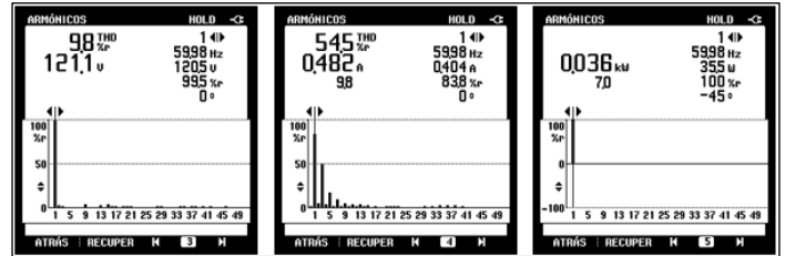
Figure 18: Harmonic components obtained by Fluke 43B analyzer in multilevel inverter with inductive-resistive load. Source: Authors, (2021).
