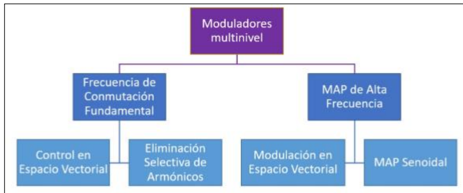
Figure 4: Classification of multilevel modulation methods. Source: [9].
