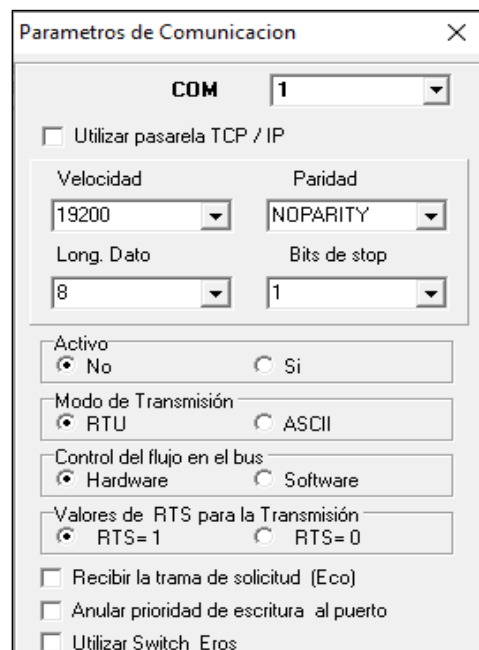
Figure 5: MODBUS MASTER configuration in Eros.
