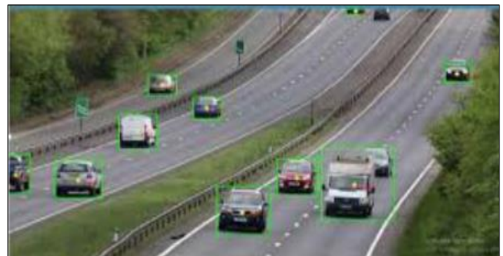
Figure 6: Detecting moving vehicles. Source: Authors, (2020).
