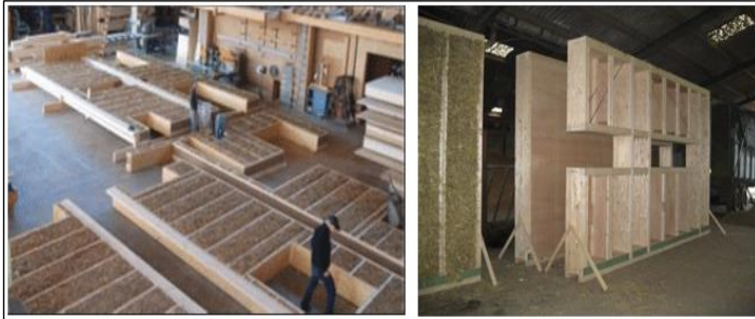
Figure 4: Straw - prefabrication with straw. Source: [6].
