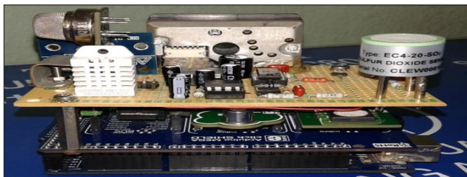
Figure 4: Photo of the prototype (The sensors can be seen on top of the shield. The Arduino can be seen below that shield.). Source: Authors, (2020).
