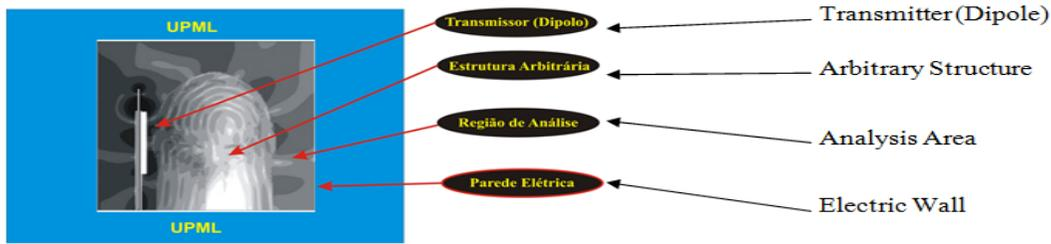
Fig 3. UPML model for the implementation of the LN-FDTD technique.
