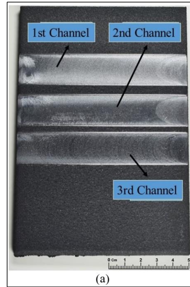
Figure 13a: Sample with sealant (nose radius 0,8 mm): (a) Machined surfaces. Source: Authors, (2022).
