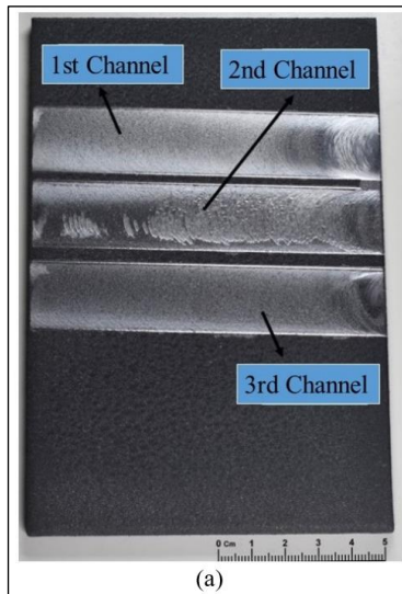
Figure 14a: Sample with sealant (nose radius 0,4 mm): (a) Machined surfaces. Source: Authors, (2022).
