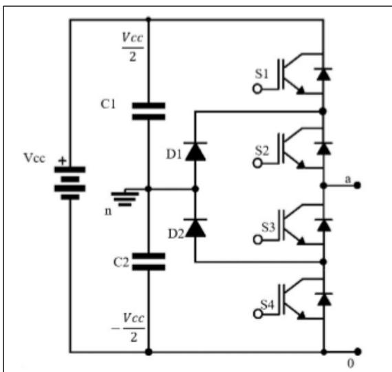
Figure 1: Three Level Anchored Diode Topology. Source: [9].
