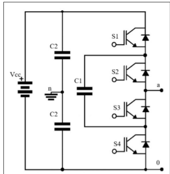
Figure 2: Inverter Topology with Three-Level Floating Capacitors. Source: [9].
