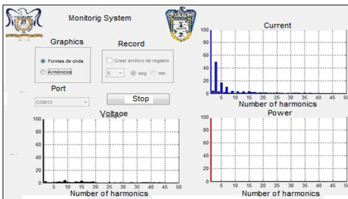
Figure 17: Harmonic components obtained through the prototype in the multilevel inverter with inductive-resistive load.
