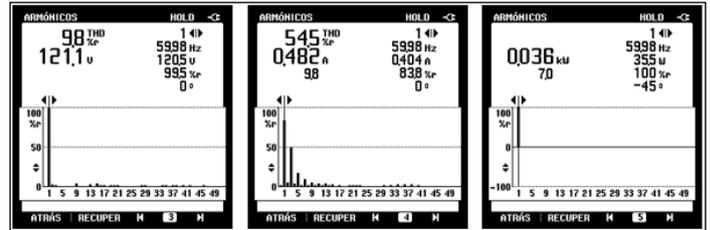
Figure 18: Harmonic components obtained by Fluke 43B analyzer in multilevel inverter with inductive-resistive load.
