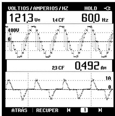
Figure 16: Waveforms Obtained by Fluke 43B Analyzer on Multilevel Inverter with Resistive Inductive Load.
