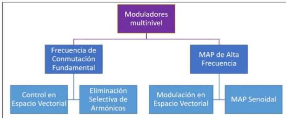
Figure 4: Classification of multilevel modulation methods. Source: [9].
