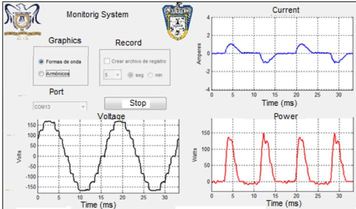
Figure 15: Waveforms obtained with the prototype in the multilevel inverter and inductive-resistive load.
