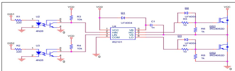
Figure 10: Conditioning circuit for trigger signals. Source: Authors, (2021).
