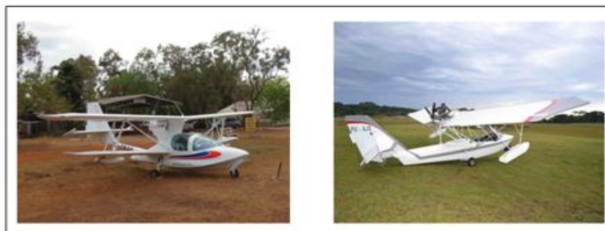
Figure 11. Super Petrel (Composite) and Corsário (Aluminum).
