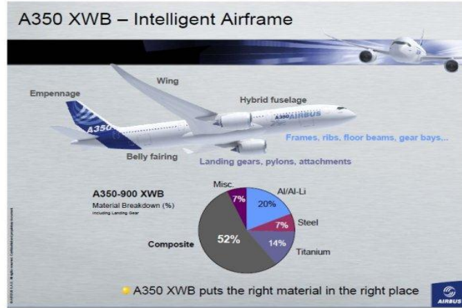
Figure 6 - Used Materials in the A350XWB Aircraft. Source: [24] .
