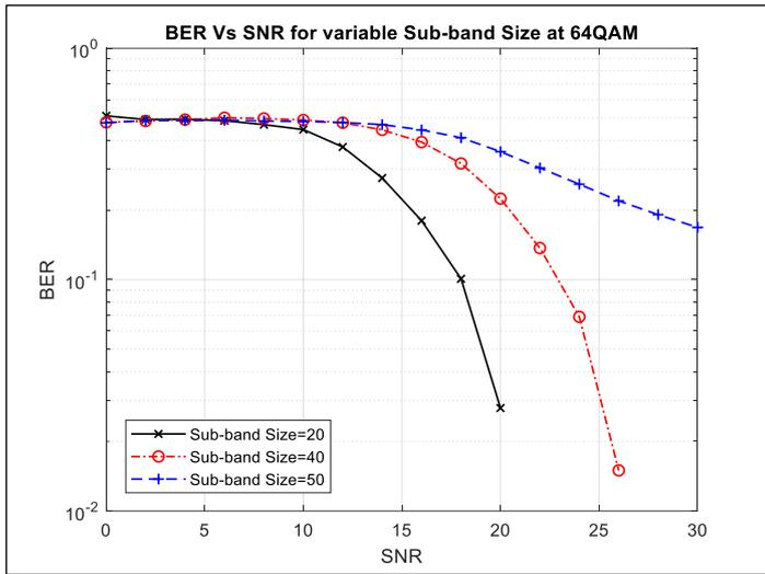
Figure 11: BER vs SNR for Polar coded UPMC Waveform with variable sub-band size. Source: Authors, (2025).
