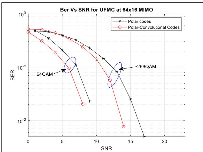
Figure 12: BER performance of joint convolutional and polar coded UPMC system with variable QAM order Source: Authors, (2025).
