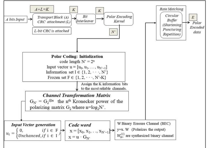
Figure 4: Polar Coding Algorithm.
