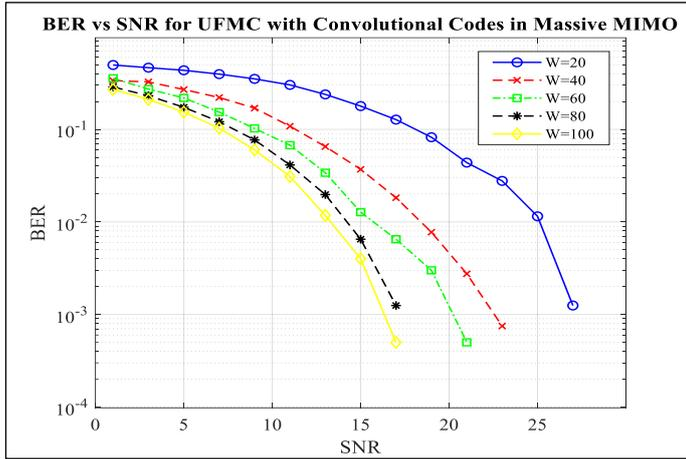
Figure 7: BER Performances for UPMC with Convolutional Codes with Variable gNB antenna array size
