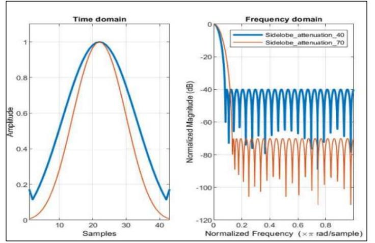
Figure 1: Time and frequency characteristics of the Chebyshev filter.
