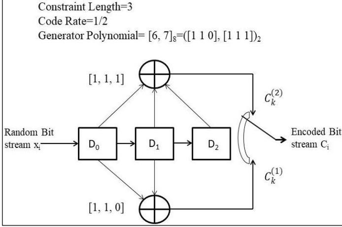
Figure 3: Convolutional Encoder.
