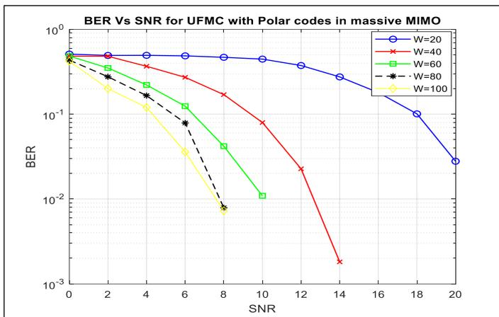
Figure 8: BER performance of Polar coded UPMC system with Variable gNB antenna array size.
