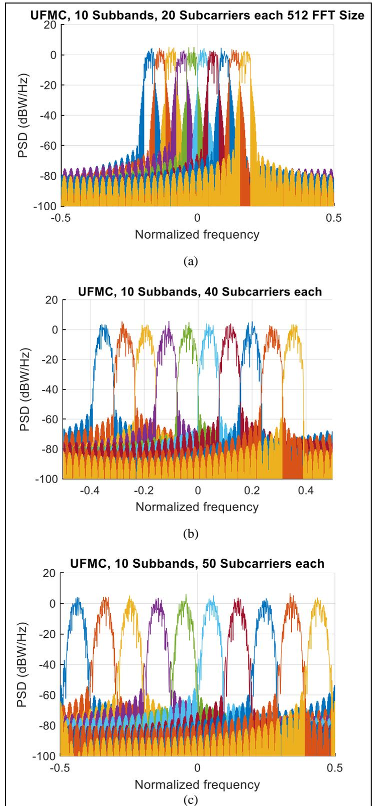
Figure 10: PSD for UPMC Waveform with (a) sub-band size=20 (b) sub-band size=40 (c) sub-band size=50.
