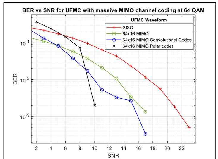
Figure 6: BER versus SNR performance of UFMC waveform with different channel codes. Source: Authors, (2025).
