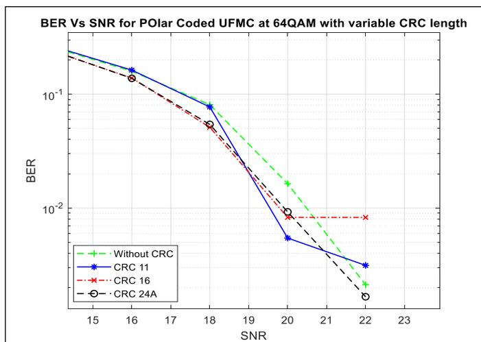
Figure 9: BER performance of Polar coded UPMC system for variable CRC length
