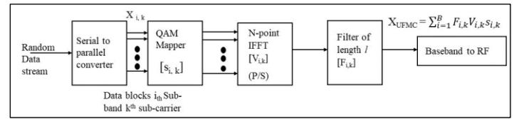
Figure 2: UFMC Modulation.
