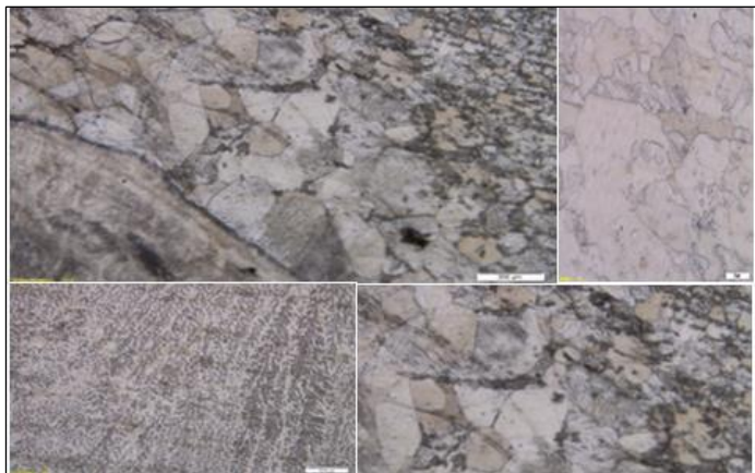
Figure 15: Sample welded at a heat input of 1.75 kJ/mm. Source: Authors, (2024).
