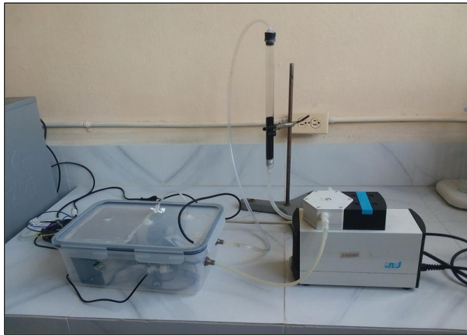
Figure 1: Experimental setup used for activated carbon adsorption.
